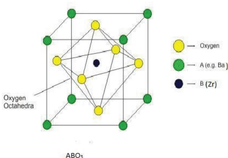
Barium zirconium titanate ceramics are attractive candidates for dynamic random access memories and tunable microwave devices. Such a lead free, environment friendly materials are known to exhibit relaxor behaviour in bulk materials with increase in Zr content. The interest in high strain materials is increasing for electromechanical transducers and various related applications.(3)
